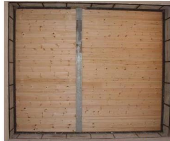
Figure 10: Sound insulation measurement according to EN 1793-2 (QUIESST, 2012)
