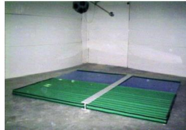
Figure 9: Sound reflection measurement according to EN 1793-1 (QUIESST, 2012)
